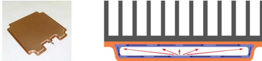
A properly designed vapor chamber with heatsink can improve the thermal performance by as much as 30% over heat pipe based solutions. It not only lowers the temperature by a number of degrees, but may eliminate the need for fans, which improves the reliability of the system and eliminates noise.
