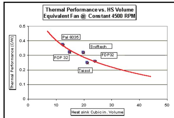
*\*The graphs above assume using aluminum as the heatsink material.*
