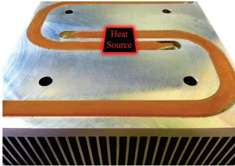
**Improve heat spreading at the heat sink base:** You can improve heat dissipation by spreading the heat across the the base of a heatsink. Embedding heat pipes within the base of a heat sink is useful in cases where there is a small concentrated heat source versus a large heat sink base.
