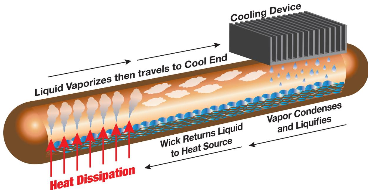
Heat pipes have become commonplace in many of today's electronics systems. Computers, video games, network equipment all rely on heat pipes for thermal management.
