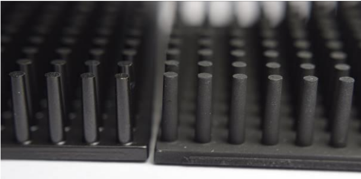
Figure 3. Close up comparison of E-Coating (Left) and Anodization (Right)
