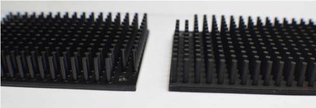
Figure 2. Side view comparison of E-Coating (Left) and Anodization (Right)
